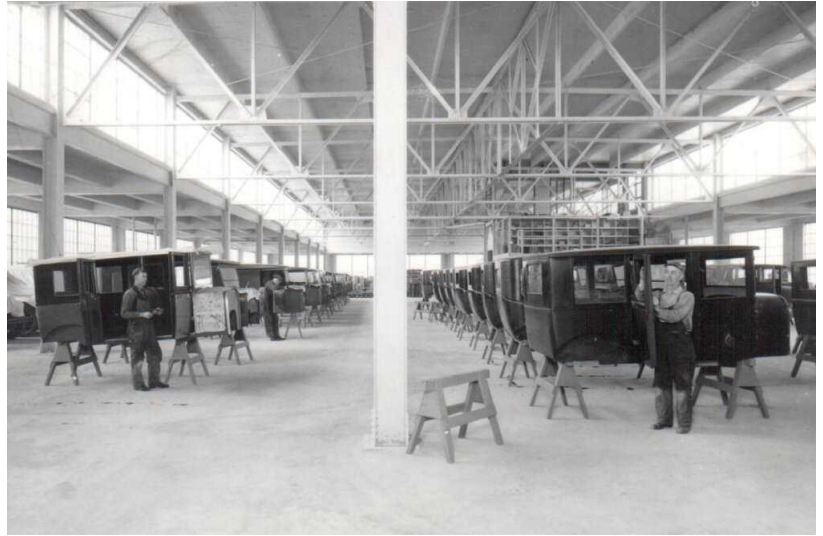
A fresh bunch of car bodies from the Fischer-Gaffeny Company are being prepared for assembly on the second floor of the Kleiber Motor Company at 10 th and Folsom St.
